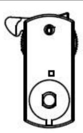
Step 3: For the lock switch, before installation, make sure it's in the status as above. Lock switch on the left.
