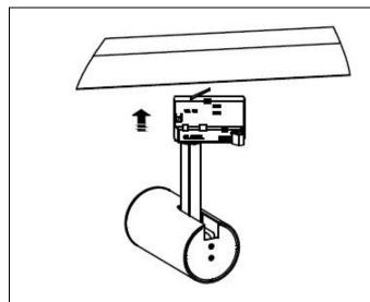
Step 1: Before commencing installation or maintenance, the electricity supply must be isolated.
