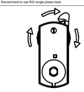
Step 4: Attach the adaptor on the track, turn the lock switch to the right as indicated.
